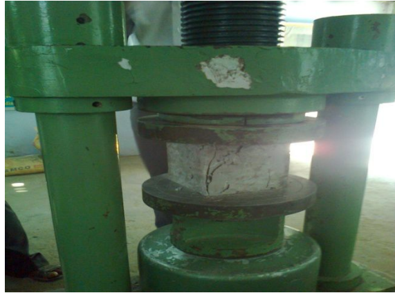
Figure 1. Determination of compressive strength of cube
