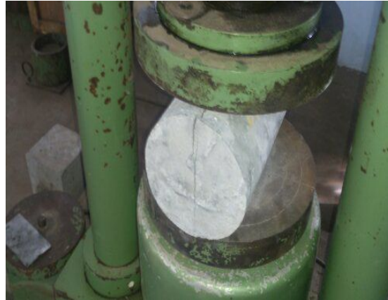
Figure 3. Determination of Split tensile strength of cube
